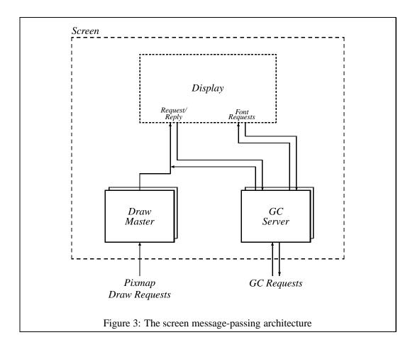
and batches drawing requests for a particular visual and depth combination; the draw masters at the screen level are used for operations on *pixmaps* (off screen rectangles of pixels). The *GC server* handles the mapping of **eXene**'s immutable pens to **X**'s mutable graphics contexts<sup>4</sup>.
