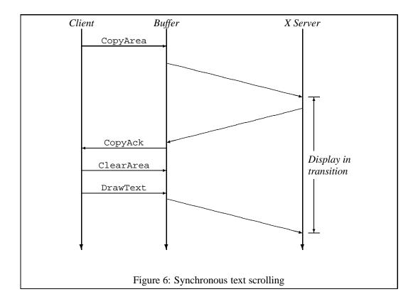
drawing operations are postponed until an acknowledgement of the copyArea is received, the period of time the display is in transition can be quite lengthy.
