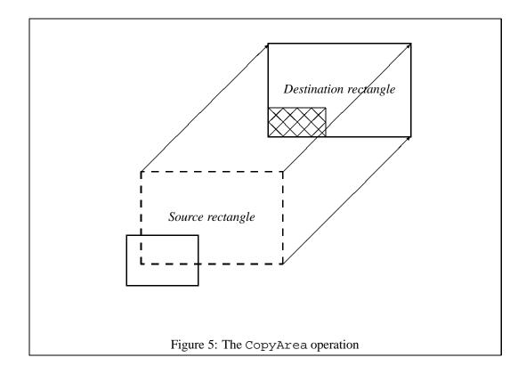
a *backing store* (or *virtual bitmap*) to handle these situations, the standard **X** policy is to notify the client that the CopyArea operation was not able to completely fill in the destination<sup>5</sup>. This policy is called *damage control*, since it is up to the client to repair the damage.
